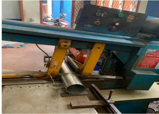
Gambar 4. 4 Pemotongan Pipa Stainless
