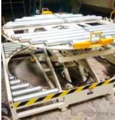
Gambar 1. 5 Lifter Pallet Conveyor
