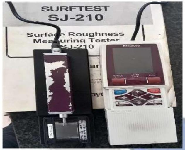
Gambar 3. 7 *Surface Roughness Tester*
