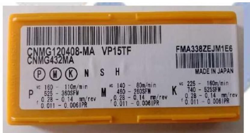
Gambar 3. 5 Pahat Potong *Insert Carbide* CNMG120408 – MA
