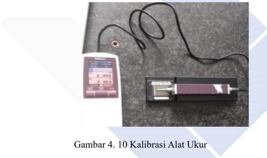
Gambar 4. 10 Kalibrasi Alat Ukur
