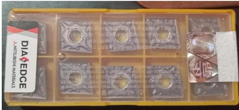
Gambar 3. 4 Pahat Potong *Insert Carbide* CNMG120404 – MA
