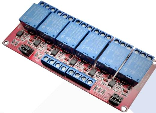
Gambar 2. 9 Relay 6 *Channel*
