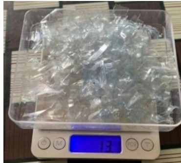
Gambar 4. 58 Penimbangan material plastik PET
