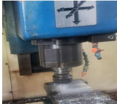
Gambar 4. 43 Facing permukaan Core
