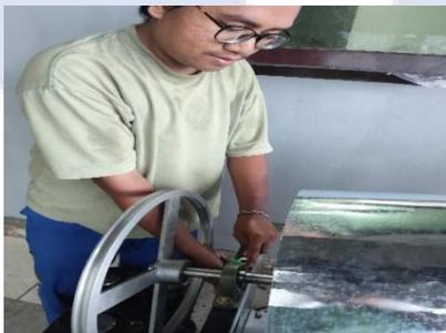
Gambar 4.9 Proses Pemasangan *Pillow Block*
