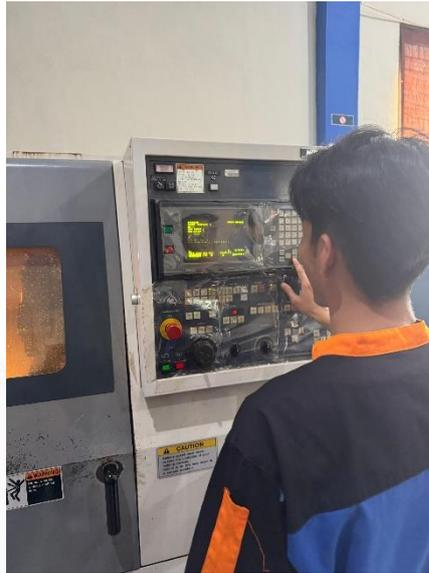
Gambar 3. 10 Proses Input Program CNC
