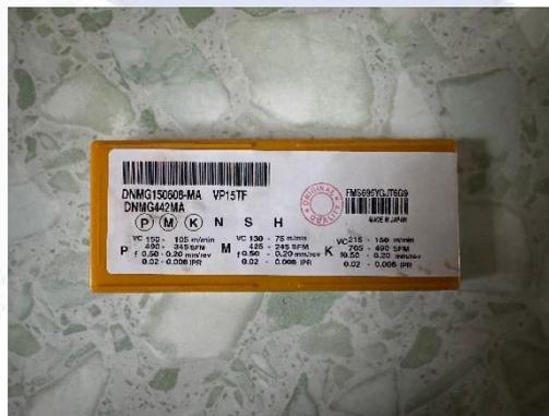
Gambar 3. 5 Mata Potong Insert Carbide DNMG 150608-MA
