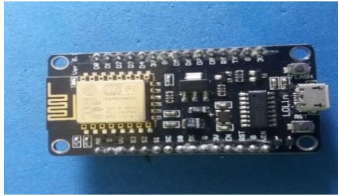
Gambar 2. 5 Module Wifi Node MCU ESP 8266
