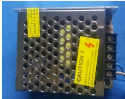
Gambar 4. 74 Power Supply 12 V 3A
