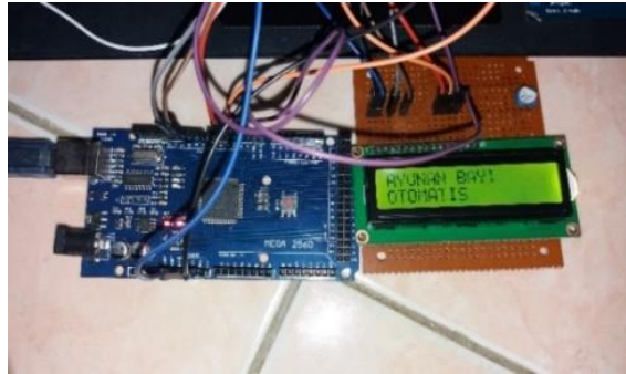
Gambar 4. 35 Hasil Uji Coba LCD 2x16
