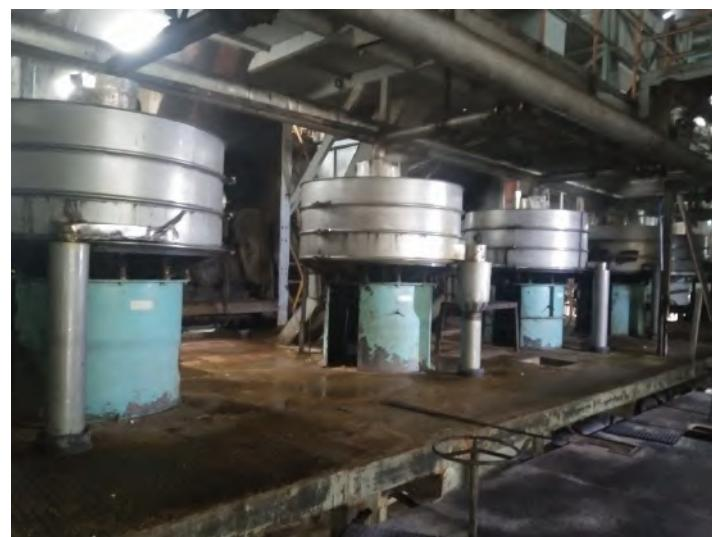
Gambar 2. 15 *Vibrating Screen DCO*
