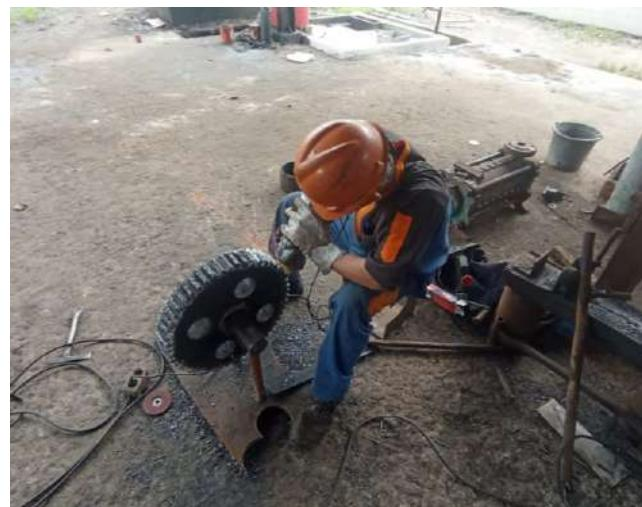
Gambar 2. 10 Merekon *Gear Band Crusher*
