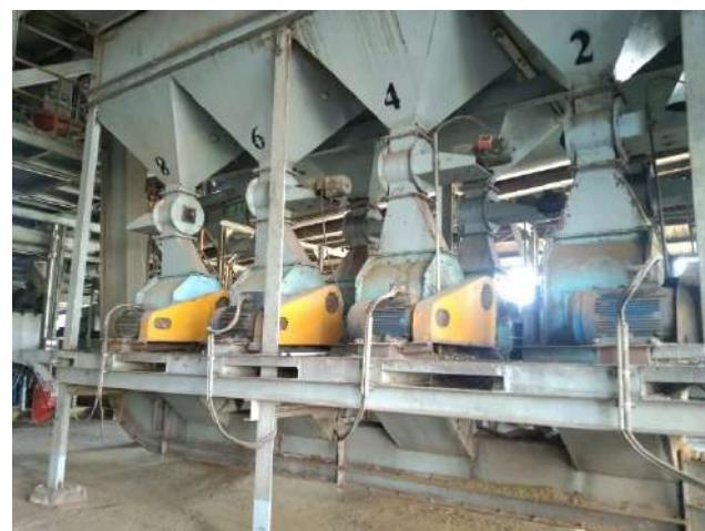
Gambar 2. 29 *Ripple Mill*
