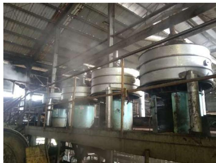
Gambar 2. 17 *Vibrating Screen Sludge*
