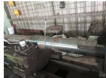
Menambal *CS conveyor*, proses permesinan bubut *roller thresher*, bubut shaft
