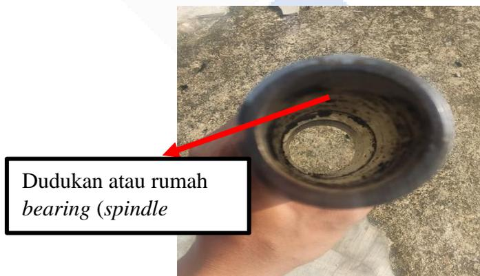
Gambar 4. 17 Rumah bearing (*spindle sleeve*)
