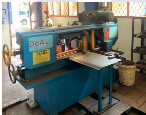
Gambar 3. 2 Mesin gergaji potong DOALL Model C-916
