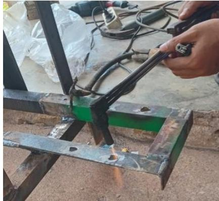
Gambar 4.17 Proses Pelubangan Dengan Cuting Tos
