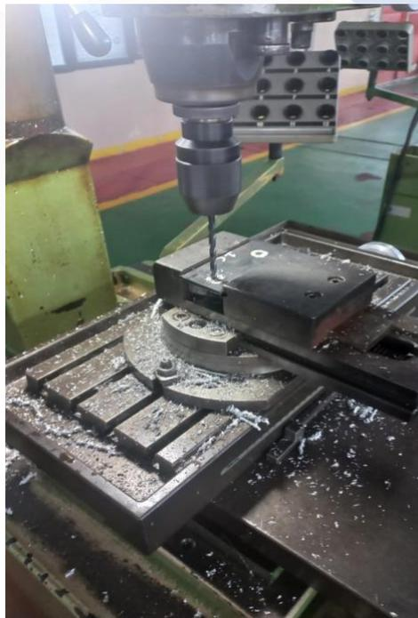
Gambar 4.6 Proses frais *braket caliper 2*
