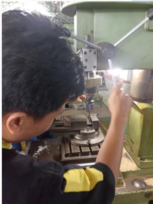
Gambar 4.5 Proses frais *braket caliper 1*
