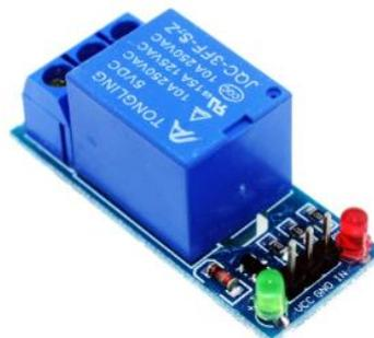
Gambar 2.6 *Relay Switch*
