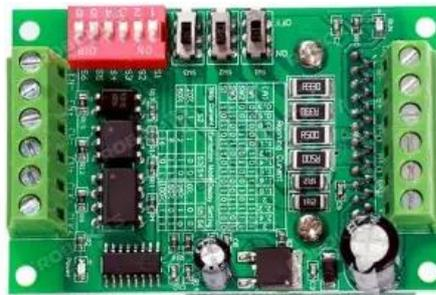
Gambar 2. 9 *Driver* Motor *Stepper* TB6560
