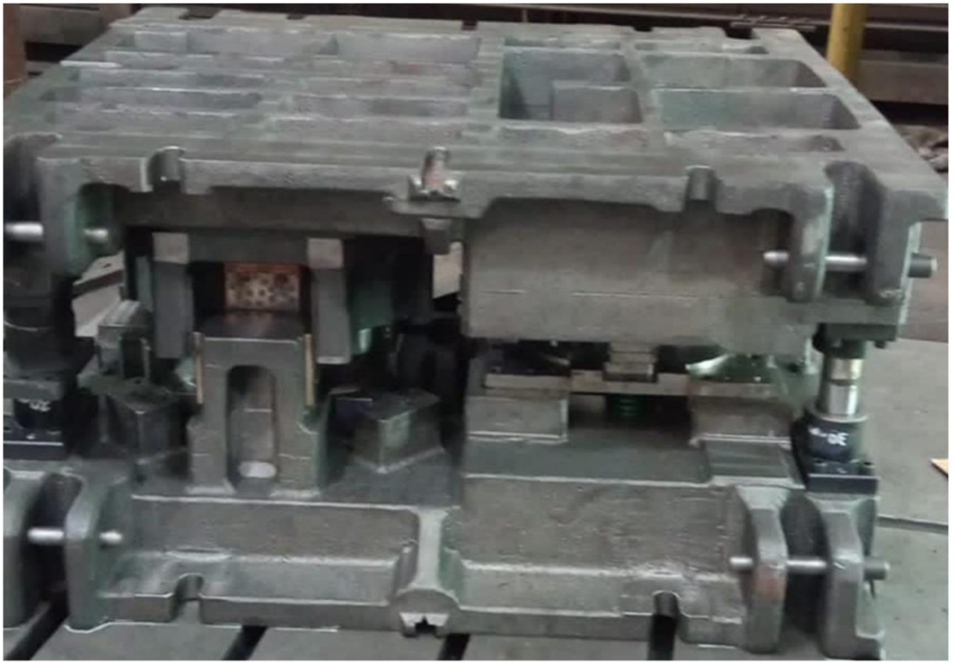
Gambar 2.9 DIES UPPER LOWER HASIL PROSES SPOTTING
