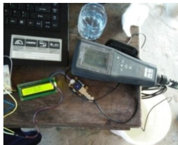
Gambar 4.34 Hasil Pengujian Sensor DO ( Dissolved Oxygen ) meter
