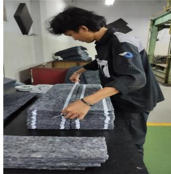
Gambar 2. 2 Proses Assy *Double Tape*
