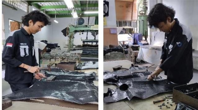
Gambar 2. 3 Proses *Punch Hole Carpet J-Series*
