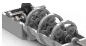
Gambar 2. 14 *Planetary Gearbox*
