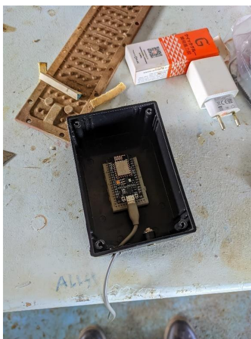
Gambar1.35 rangkaian system panic button berbasis esp8266
