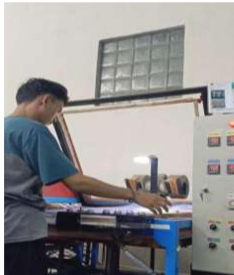
Gambar 2. 2 Proses Vakum Service Hole
