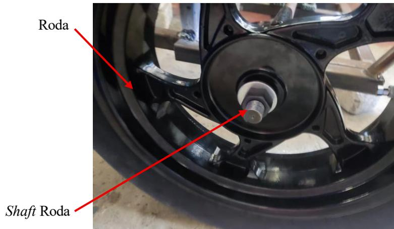
Gambar 4. 15 Proses Pemasangan Ban Kedalam *Shaft* Roda
