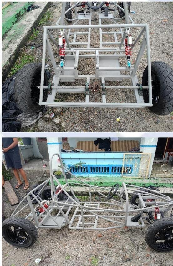
Gambar 4. 16 Proses Assembly Rangka Bagian Belakang
