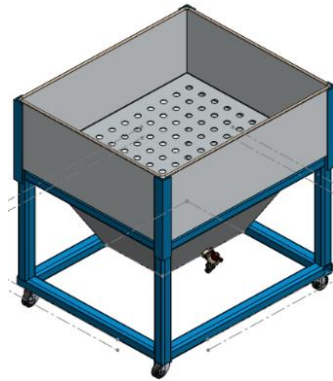
Gambar 2. 7 Desain bak pallet
