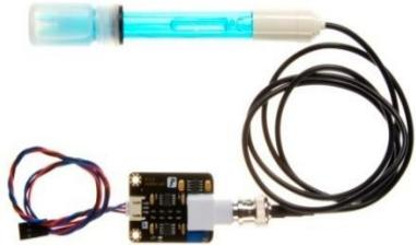
Gambar 2.3 Sensor pH air [11]
