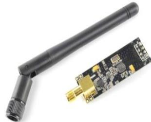
Gambar 2.5 NRF24L01 *Module Wireless* [14]
