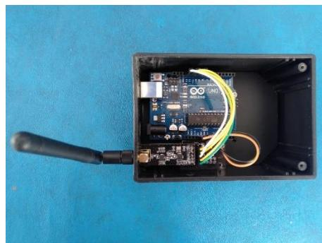
Gambar 4.19 *Hardware Elektrik Receiver*
