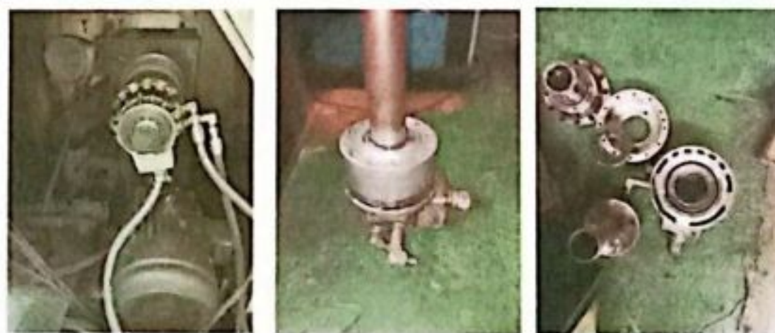
Gambar 2. 14 Proses penggantian seal Hidolik cylinder clamp chuck.
