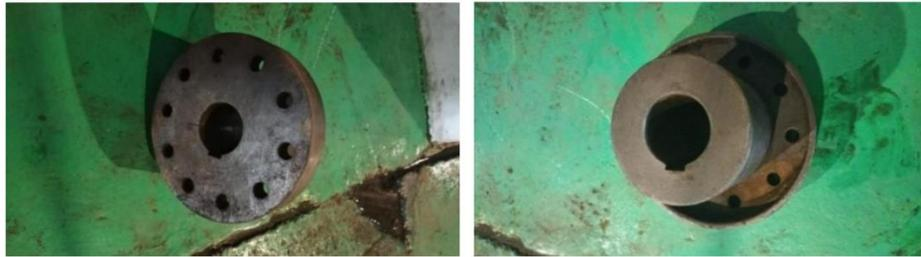
*Gambar 10 2.2 Coupling Pompa*
