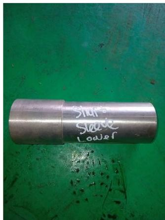
*Gambar 21 2.13 Lower Shaft Sleeve*
