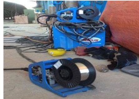
Gambar 1.10 Mig Arc Welding Steel/Alumunium
