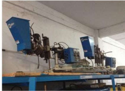
Gambar 1.9 Submerged Arc Welding
