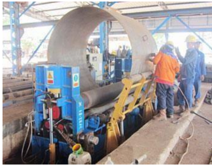
Gambar 1.6 Plate Rolling Machine
