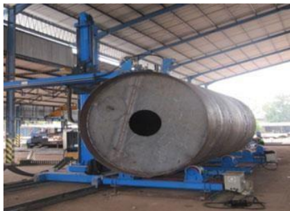
Gambar 1.8 Auto Welding Manipulator Machine
