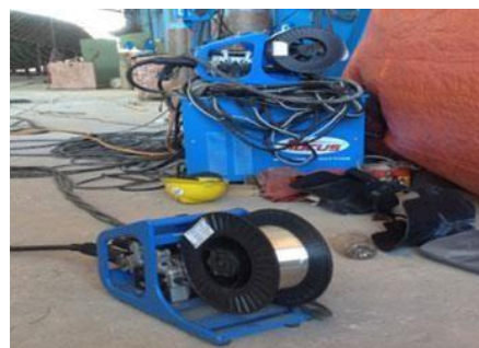
Gambar 1.11 Mig Arc Welding Steel/Alumunium
