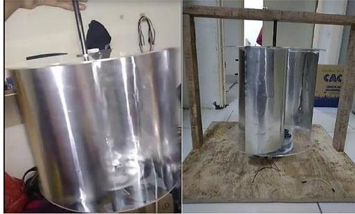
*Gambar 2. 3 Design of Savonius model wind turbine for power catchment [4]*
