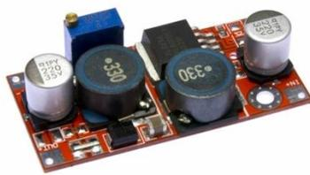
*Gambar 2. 11 Buck Boost Converter*
