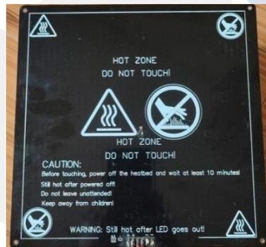
Gambar 2. 7 *Heat Bed* 3D Printer
