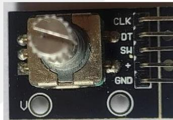
Gambar 2. 10 Rotary Encoder
