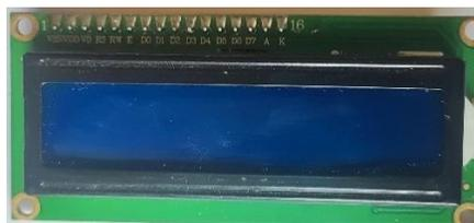
Gambar 2. 9 LCD 2 x 16
