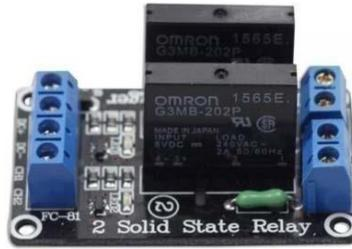
**Gambar 2. 4 Modul Relay Solid State(Suryono2022).**
