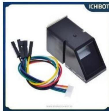
Gambar 2. 3 Sensor *Fingerprint* AS608
