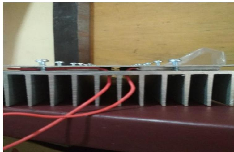
Gambar 4.19 Tampilan Sirip *Heatsink*
