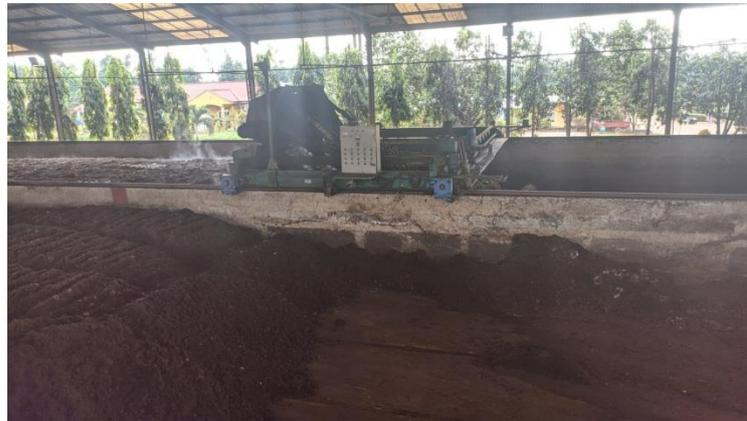
Gambar 6 Mesin *Turner plant 2*
