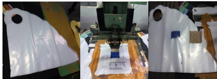
Gambar 2. 1 Proses Welder Service Hole
