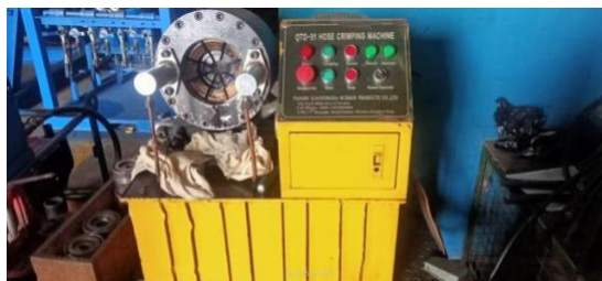
Gambar 2. 7 Crimping hose machine
