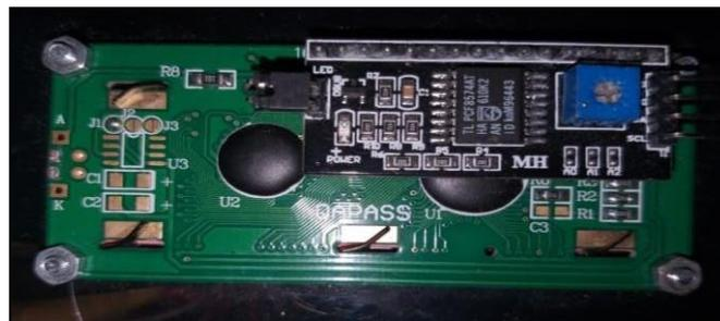
Gambar 2.7 LCD 16 x 2
