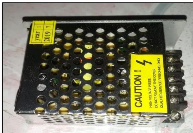
Gambar 2.10 *Switch – Mode Power Supply* 12V
