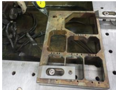
Gambar 2.8 Proses setting material
