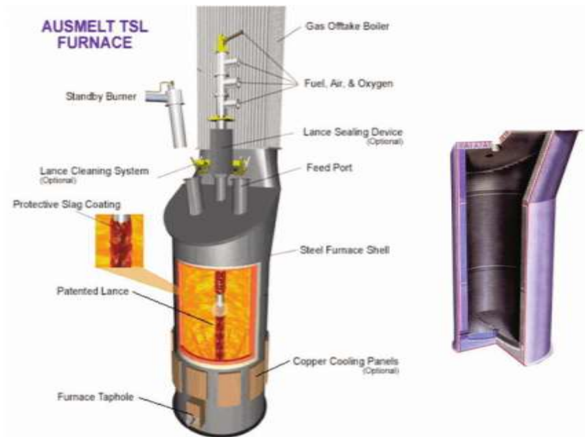
Gambar 1.4 Ausmelt Furnace in operation [left] section of reactor [right]
