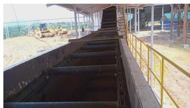
Gambar 2. 2 *FFB Inclined Scraper*
