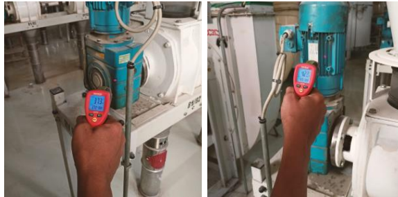
Gambar 2. 8 Mengecek suhu Gearbox dan Motor
