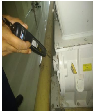
Gambar 2. 3. Mengecek Suara Bearing Airlock
