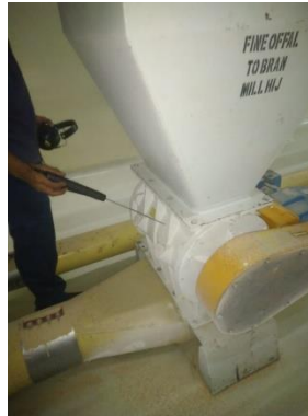
Gambar 2. 5. Mengecek suara body airlock
