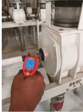
Gambar 2. 2. Mengecek suhu bearing airlock
