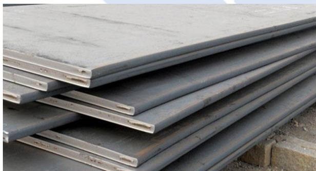
Gambar 2.1. Plat ASTM A36
