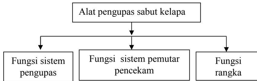
Gambar 4.2 Diagram Sub Fungsi Bagian.
