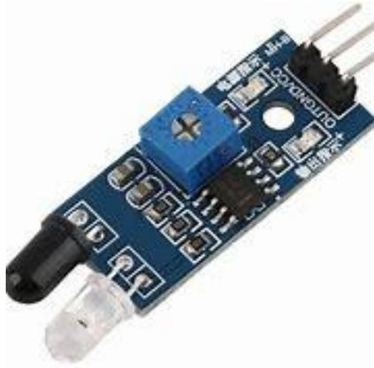
Gambar 2.7 Sensor Infrared
