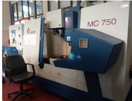
Gambar 3.4 CNC Milling Lagun MC-750
