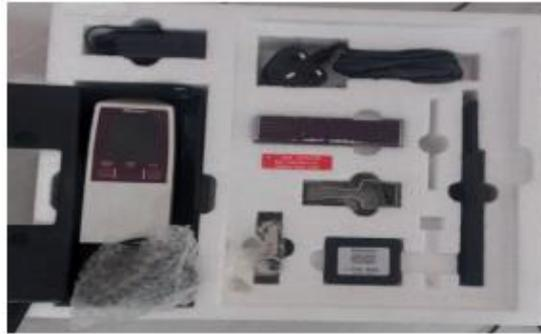
Gambar 3.4 Surface Roughness Tester type Mitutoyo SJ-210
