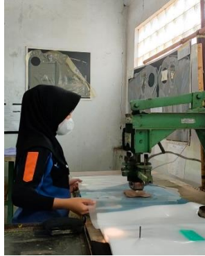
Gambar 2. 4 Proses Assy Welder Sub Sheet
