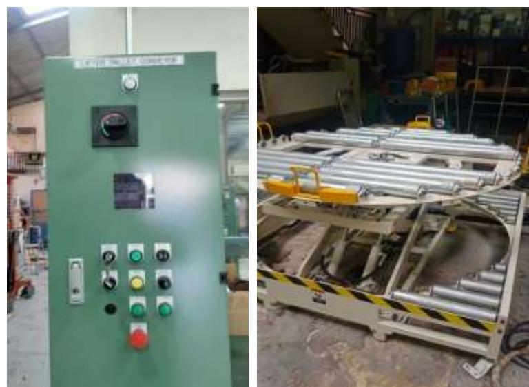
Gambar 1. 12 Lifter Pallet Conveyor
