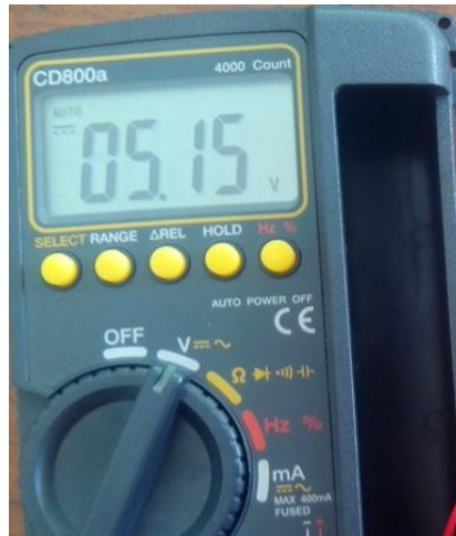
Gambar 4.9 Hasil pengujian Power Supply 5v 3A
