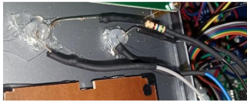
Gambar 4.30 Pemasangan led indikator
